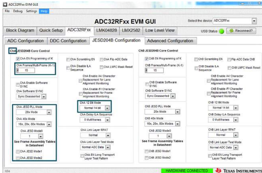
Figure 20. ADC32RFxx-EVM GUI JESD204B Configuration Tab DDC Mode
