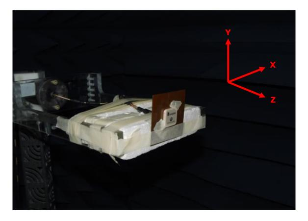
The antenna is measured on a CTIA certified anechoic chamber. The CGIP.25 antenna is put on a 70\*70mm ground plane.
