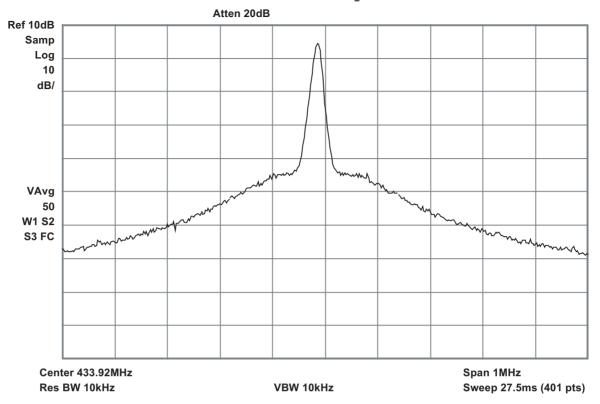
Figure 3-9. FSK-modulated TX Spectrum (433.92MHz/20Kbit/s/±16.17kHz/Manchester Code)
