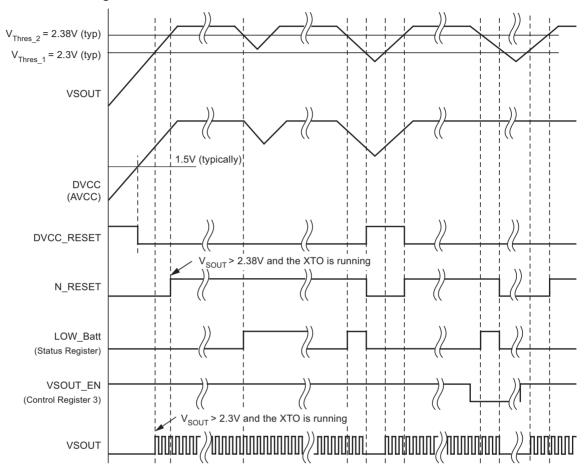
Figure 5-4. Reset Logic, SR Latch Generates the Hysteresis in the NRESET Signal
