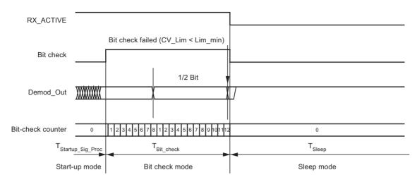
Figure 9-7. Timing Diagram for Failed Bit Check (Condition: CV\_Lim ≥ Lim\_max)
