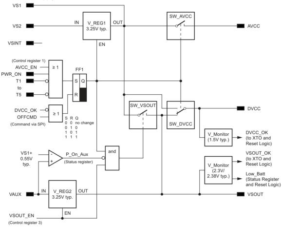
The supply voltage range of the ATA5428 is 2.4V to 3.6V or 4.4V to 6.6V.
