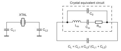
With  $C_m \le 14fF$ ,  $C_0 \ge 1.5pF$ ,  $C_{LN} = 9pF$  and  $C_L = 7.4pF$  to 10.6pF, the pulling amounts to  $P \le \pm 100ppm$  and with  $C_m \le 7fF$ ,  $C_0 \ge 1.5pF$ ,  $C_{LN} = 9pF$  and  $C_L = 7.4pF$  to 10.6pF, the pulling is  $P \le \pm 50ppm$ .
