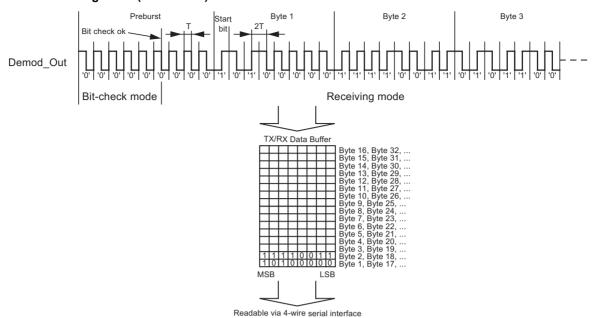
If the TX/RX data buffer control logic detects a bit error, an interrupt is issued and the transceiver is set back to the start-up mode (see Figure 9-1 on page 46, Figure 9-2 on page 47 and Figure 9-10).
