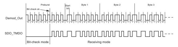
If the transparent mode is inactive (T\_MODE = 0), the received data stream is buffered in the TX/RX data buffer (see Figure 9-9 on page 52). The TX/RX data buffer is only usable for Manchester and Bi-phase coded signals. It is always possible to transfer the data from the data buffer via the 4-wire serial interface to a microcontroller (see Figure 8-1 on page 41).
