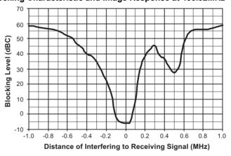
This high blocking performance even makes it possible for some applications using quarter wave whip antennas to use a simple LC band-pass filter instead of a SAW filter in the receiver.
