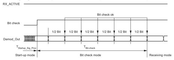
As seen in Figure 9-4, the time window for the bit check is defined by two separate time limits. If the edge-to-edge time  $t_{ee}$  is in between the lower bit-check limit  $T_{\text{Lim\_min}}$  and the upper bit-check limit  $T_{\text{Lim\_max}}$ , the check will be continued. If  $t_{ee}$  is smaller than limit  $T_{\text{Lim\_min}}$  or exceeds  $T_{\text{Lim\_max}}$ , the bit check will be terminated and the transceiver switches to sleep mode.
