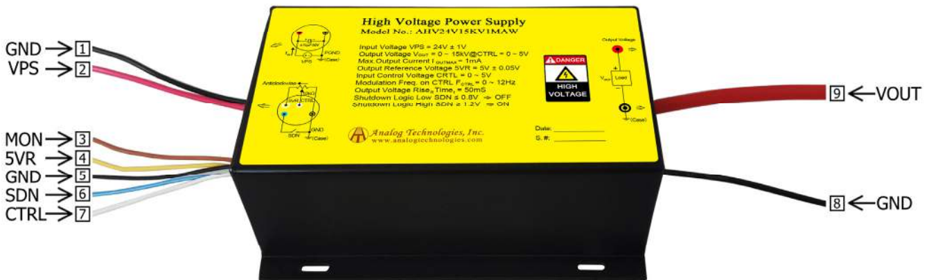
Figure 2. The Connecting Lead Wires of AHV24V15KV1MAW
