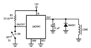
\*\*\* To assure shutdown, select Resistor R3 to ensure at least 300µA of pull-up current when S1 is open. (Assume 2V at the ON/OFF pin.)
