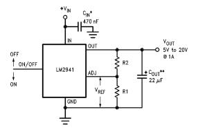
$$\begin{split} &V_{OUT} = \text{Reference voltage} \times \frac{\text{R1} + \text{R2}}{\text{R1}} \text{ where } V_{REF} = 1.275 \text{ typical} \end{split}$$
