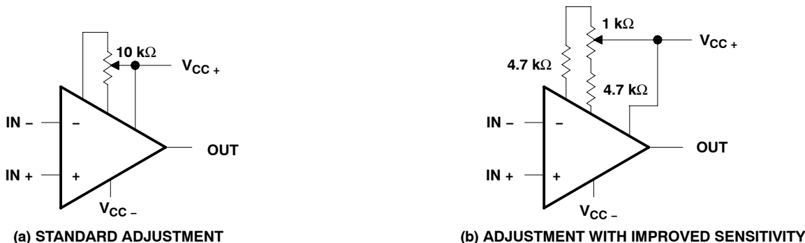
Figure 55. Input Offset Voltage Nulling Circuits
