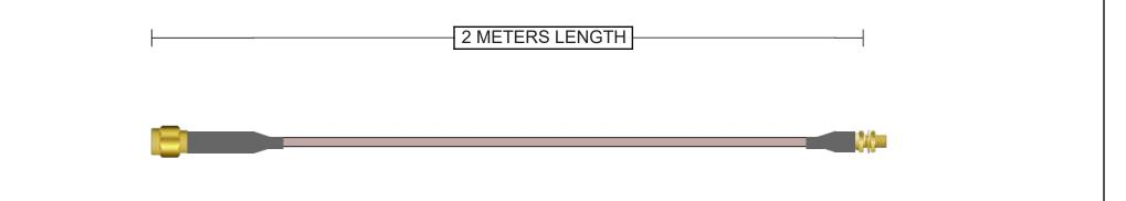
Connector A 132114RP SMA Plug Straight Brass Gold + Heatshrink 50 Ohm RG-316 Continuity/Hi-Pot
