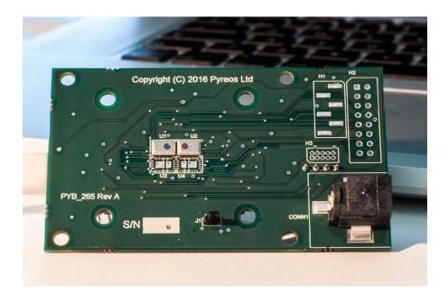
The Broadcom<sup>®</sup> ezPyro<sup>™</sup> application-specific evaluation kits demonstrate the capabilities of Broadcom's innovative ezPyro digital SMD infrared sensors. The evaluation kits consist of a main board with up to four ezPyro sensors and an attached controller board based on an ARM Cortex-M4 microcontroller. There are specific kits for gas, flame, motion, and gesture sensing, as well as a generic kit that allows various ezPyro sensors to be plugged into a backplane board.
