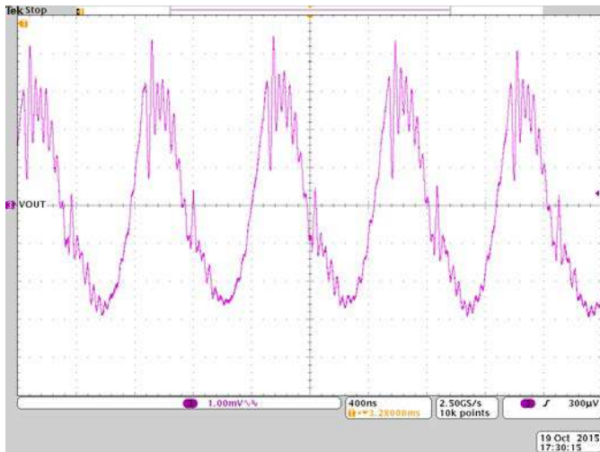
Figure 15: Output ripple V_{IN} = 5V , V_{OUT} = 3.3V
