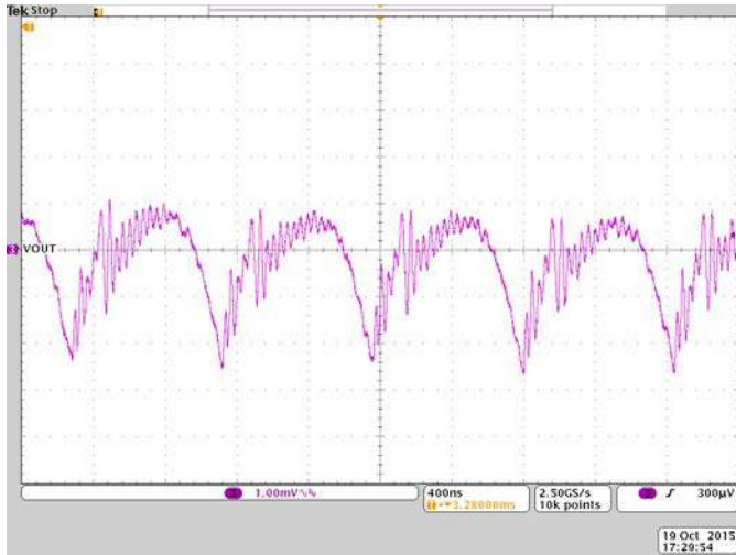
Figure 13: Output ripple V_{IN} = 5V , V_{OUT} = 1V
