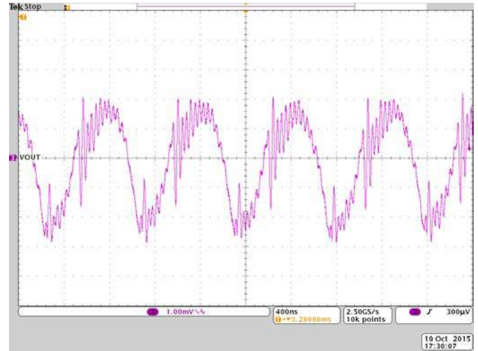
Figure 14: Output ripple V_{IN} = 5V , V_{OUT} = 1.8V
