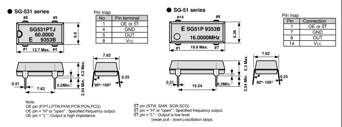
To maintain stable operation, provide a 0.01uF to 0.1uF by-pass capacitor at a location as near as possible to the power source terminal of the crystal product (between Vcc - GND).
