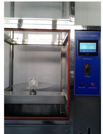
Testing under water jet
