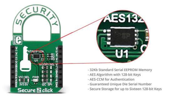
The AES-128 cryptographic engine operates in AES-CCM mode to provide authentication, stored data encryption/decryption, and Message Authentication Codes. Data encryption/decryption can be performed for internally stored data or for small external data packets, depending upon the configuration. Data encrypted by one ATAES132A device can be decrypted by another, and vice versa.
