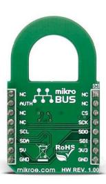
**Secure 2 click** carries the ATAES132A, a cryptographic coprocessor with secure hardware-based key storage from Microchip. The click is designed to run on either 3.3V or 5V power supply. Secure 2 click communicates with the target microcontroller over SPI and I2C interface, with additional functionality provided by the INT pin on the mikroBUS<sup>TM</sup> line. The click comes with stackable headers so you can put another click on the top of it.
