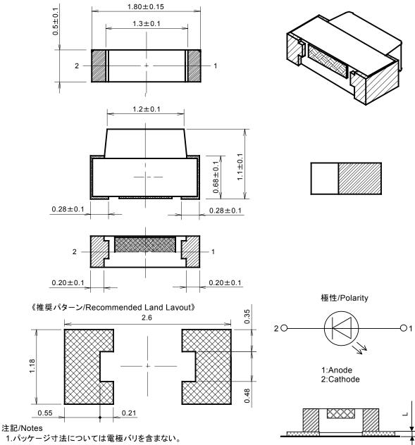
Measurement of the package doesn't include electrode projection.
