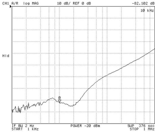
Figure 21. LDO2 PSRR vs. Frequency, V_{OUT2} = 2.85\text{ V} , I_{OUT2} = 100\text{ mA}
