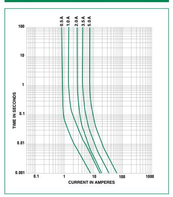
Derating depicted in this curve is in addition to the standard derating of 25% for continuous operation.
