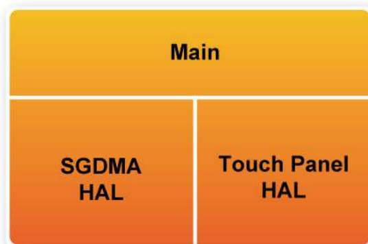
Figure 4-3 Software stack of the tPad Starter demonstration
