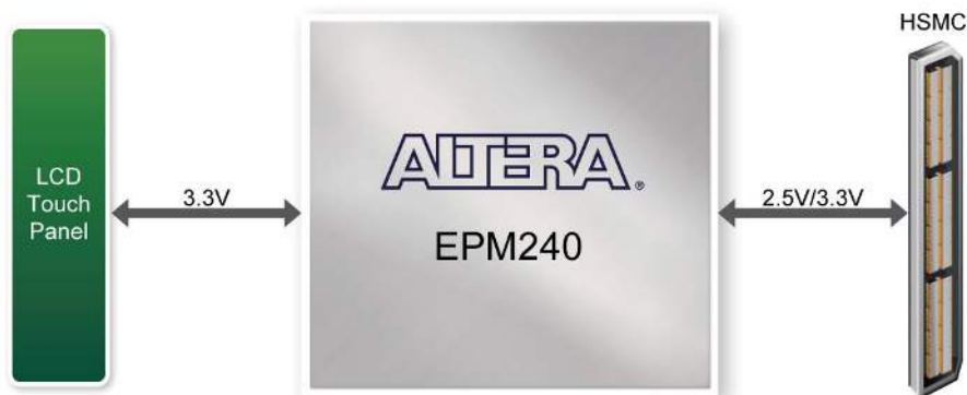
Figure 3-6 Block Diagram of the Bus Controller
