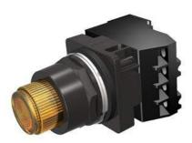
30mm BlackMax, Epoxy Coated Corrosion Resistant Complete Metal Unit PTT / Illuminated Pushbutton Transformer type, 600V AC Incandescent Lamp Extended Button Plastic Lens, Amber 2 Position Momentary with 1 N.O. - 1 N.C. Heavy Duty Contacts, A600/P600 UL Listed, CSA Certified NEMA 1,3,3R,4,4X,12,13 & Automotive Standards
