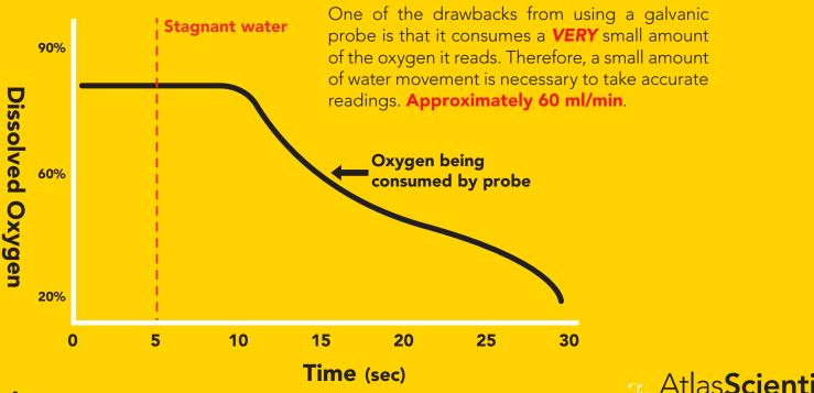
This galvanic dissolved oxygen probe is a passive device that generates a small voltage from 0mv - 60+mv depending on the oxygen saturation of the PTFE sensing membrane. This voltage can easily be read by a multimeter or an analog to digital converter.
