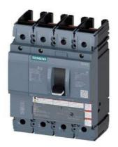
circuit breaker 3VA5 UL frame 250 breaking capacity class C 100kA @ 480V 4-pole, line protection TM230, FTAM, In=90A overload protection Ir=90A fixed short-circuit protection Ii=5...10 x In N conductor unprotected without connection
