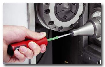
TorqueVario-S ESD was developed for use in anti-static environments and TorqueVario-S provides safety when working with electrical components. All Wiha TorqueVario-S models have an integrated window scale that displays the torque value - a completely new design, which eliminates false readings. The torque value is continuously adjustable by using the provided adjustment tool (TorqueSetter) this prevents the setting from being altered unintentionally.
