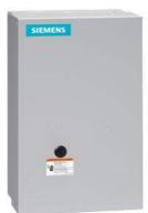
Non-reversing contactor, Size 3 1/2, Three phase full voltage, Contactor amp rating 115A, 3 wire (NO aux included), 24VAC 50-60Hz coil, Non-combination type, Enclosure NEMA type 1, Indoor general purpose use, Standard width enclosure
