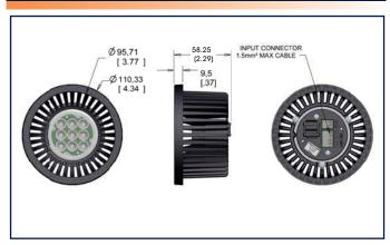
Diameter x H 110.33mm x 58.25mm (4.34" x 2.29") Maximum Cable Dia - 1.5mm<sup>2</sup> / 16 AWG
