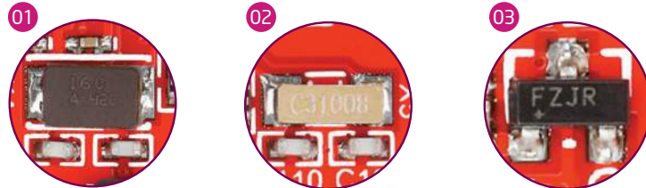
Figure 5-1: Crystal oscillator and 2.048V reference
