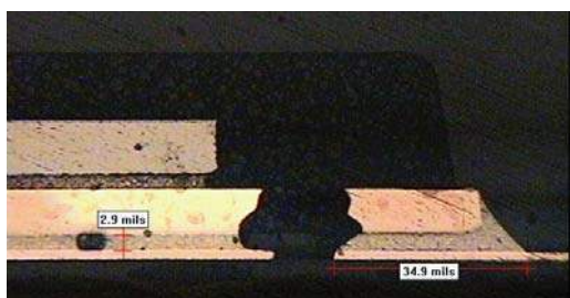
50% Paste Coverage, Plugged Via, 2.9 mil Standoff
