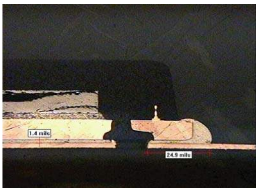
37% Paste Coverage, Plugged Via, 1.4 mil Standoff
