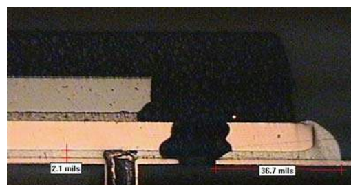
81% Paste Coverage, Encroached Via, 2.1 mil Standoff
