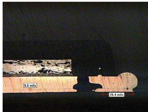
37% Paste coverage, Encroached Via, 0.6 mil Standoff
