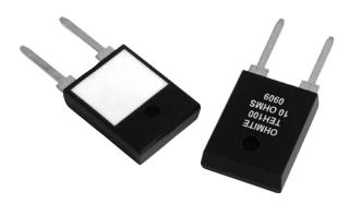
Ohmite offers the totally encapsulated and insulated TO-247 package for low ohmic value and non-inductive design for high-frequency and pulsing applications. Ideal use is for power supplies. This series is rated at 100 Watts mounted to a heat sink.
