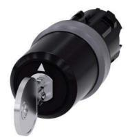
Key-operated switch BKS, 22 mm, round, plastic with metal front ring, lock No. E9 (VW), without key, 3 switch positions I-O-II, latching, actuating angle 2x45°, 10:30h/12h/13:30h, Key removal I+O+II, with laser labeling, upper case and lower case, always upper case at beginning of line
