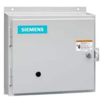
Non-reversing NEMA contactor, Size 1, Three phase full voltage, Contactor amp rating 27A, 3 wire (NO aux included), 380-440/440-480V 50/60Hz coil, Non-combination type, Enclosure NEMA type 12, Dust/drip proof for indoors, Standard width enclosure
