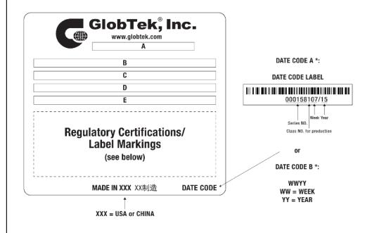
A=ICT/ITE Power Supply B=P/N: (料号) WR95E2000LCP-F(R6B) C=Model (型号) GT-86240-2412-W2U D=Input (输入)100-240V~, 50-60Hz, 1A E=Output (输出)12.0 V == 2.0 A, 24.00W
