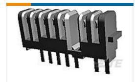
TE Part #1827684-1 2mm pitch Battery Rec. Assy. 7Pos. H = 4.0
