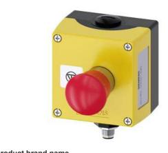
Enclosure for command devices, 22 mm, round, enclosure material metal, Enclosure top part yellow, 1 control point metal, A=Emergency stop mushroom pushbutton red, 40 mm, rotate-to-unlatch, 2 NC, spring-loaded terminal, floor mounting, silver label, black font, with graphic symbol: Emergency stop, M12 connector (5-pin) bottom, insulated reserve conductors Label glued in
