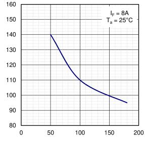
RATE OF CHANGE OF CURRENT :  $di/dt(A/\mu s)$  di/dt-tfr CHARACTERISTICS
