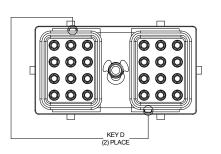
24 POS, PLUG, SOCKET, ARC SERIES, KEYED, NORMAL SEAL, BLACK
