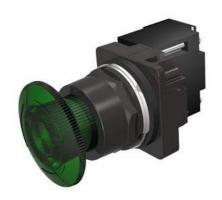
30mm BlackMax, Epoxy Coated Corrosion Resistant Metal Operator, Round Illuminated Twist-to-Release Transformer type, 240V AC Incandescent Lamp Mushroom Head Cap Small 1.79" (45 mm) Plastic Cap, Green 2 Position Maintained, Twist-to-Release UL Listed, CSA Certified NEMA 1,3,3R,4,4X,12,13 & Automotive Standards
