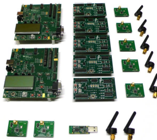
Figure 1 - CC2530 ZigBee Development Kit Contents
