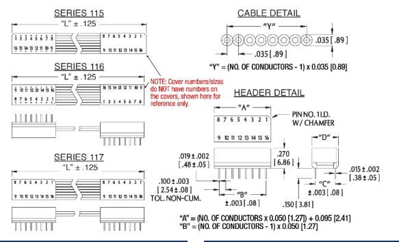
ALL DIMENSIONS: INCHES [MILLIMETERS] ALL TOLERANCES: ±0.005 [0.13] UNLESS OTHERWISE SPECIFIED CONSULT FACTORY FOR OTHER SIZES AND CONFIGURATIONS CUSTOMIZATION: ARIES SPECIALIZES IN CUSTOM DESIGN AND PRODUCTION. SPECIAL MATERIALS, PLATINGS, SIZES, AND CONFIGURATIONS CAN BE FURNISHED, DEPENDING ON QUANTITY.
