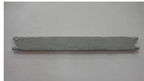
Thermal glue on rear surface
