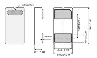
Note)The applicable specification describes in detail for SMD1006. This figure is only for reference.
