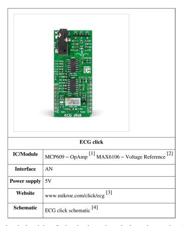
ECG click measures the electrical activity of a beating heart through electrodes taped to the skin. It requires little setup, and the final measurement results can be displayed as an Electrocardiogram using a free app.
