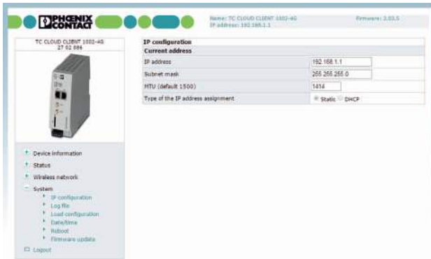
Figure 17 System, IP configuration
