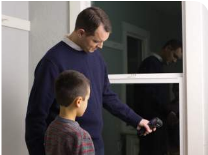
See where heat is lost through windows or doors
