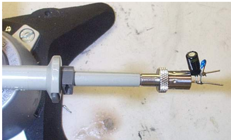
Figure 21 – Oscilloscope Probe with Probe Master ( www.probemaster.com ) 4987A BNC Adapter. (Modified with wires for ripple measurement, and two parallel decoupling capacitors added)
