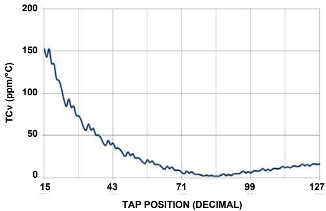
FIGURE 13. 10kΩ TCv vs TAP POSITION, V_{CC} = 3.3V
