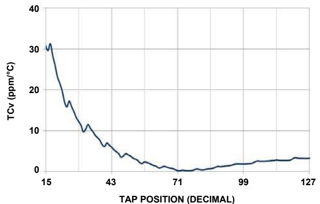
FIGURE 14. 50kΩ TCv vs TAP POSITION, V_{CC} = 3.3V
