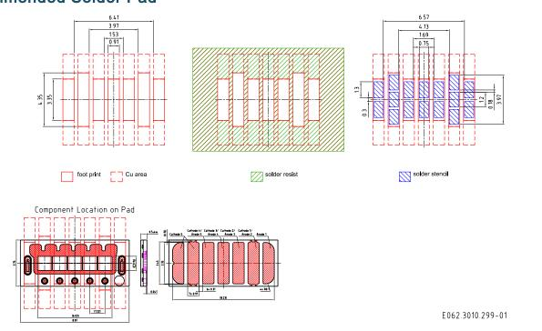
For superior solder joint connectivity results we recommend soldering under standard nitrogen atmosphere. Package not suitable for ultra sonic cleaning. To ensure a high solder joint reliability and to minimize the risk of solder joint cracks, the customer is responsible to evaluate the combination of PCB board and solder paste material for his application.
