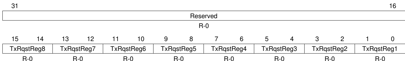
Figure 24-28. Transmission Request X Register (DCAN TXRQ X) [offset = 84h]
