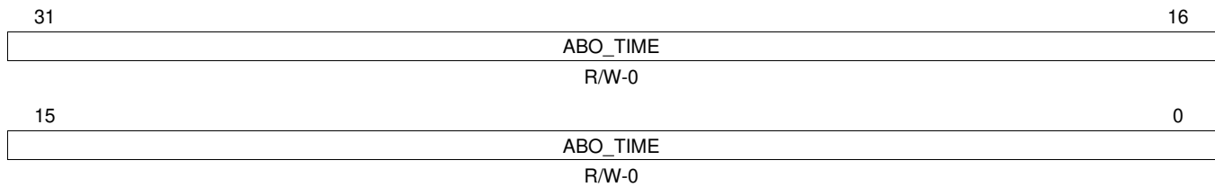
Figure 24-27. Auto-Bus-On Time Register (DCAN ABOTR) [offset = 80h]
