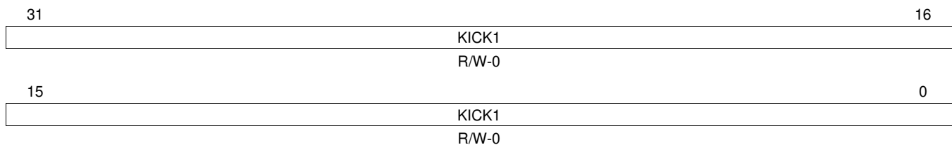
Figure 4-7. KICK_REG1: Kicker Register 1 (Address = FFFFEA3Ch)
