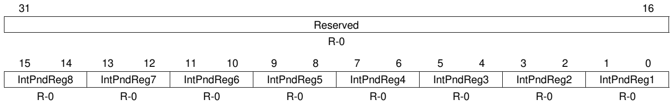
Figure 24-38. Interrupt Pending X Register (DCAN INTPND X) [offset = ACh]
