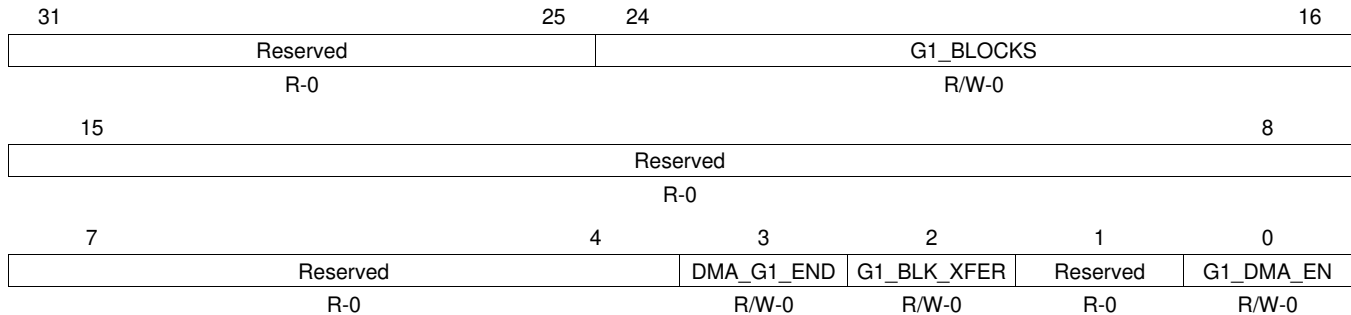
Figure 19-41. ADC Group1 DMA Control Register (ADG1DMACR) [offset = 50h]
