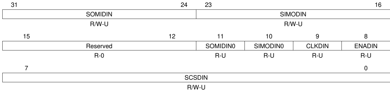
Figure 25-33. SPI Pin Control Register 2 (SPIPC2) [offset = 1Ch]
