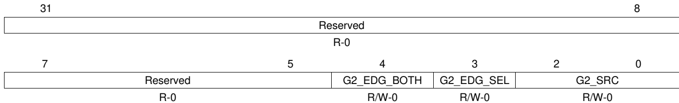
Figure 19-30. ADC Group2 Trigger Source Select Register (ADG2SRC) [offset = 24h]
