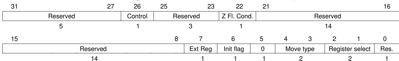
Figure 20-154. MOV32 Control Field (C31:C0)
