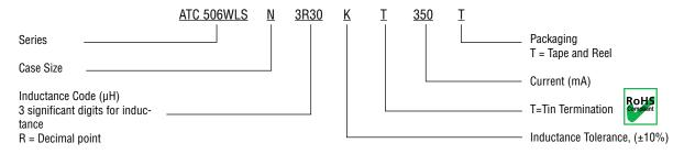
The above part number refers to a 506WLS Series, Case Size N, 3.30 µH inductor, K tolerance (±10%, typ.), with Tin Termination(T), 350 mA, tape and reel packaging.
