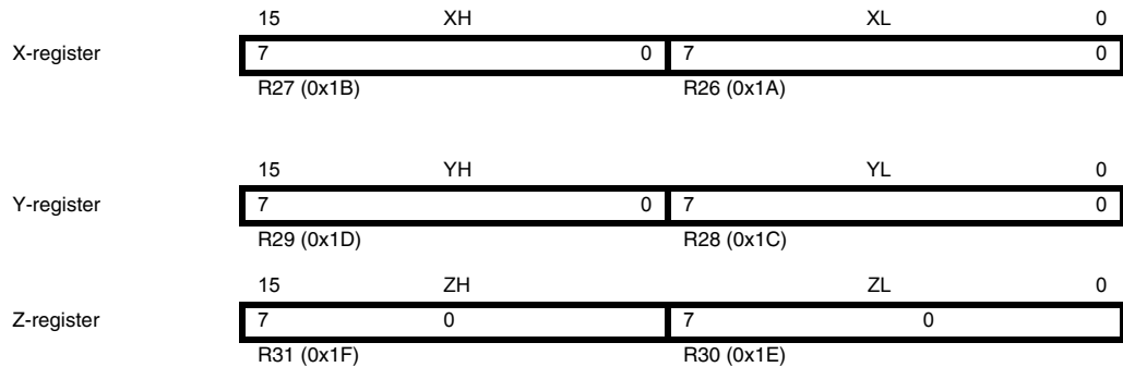
Figure 7-3. The X-, Y-, and Z-registers
