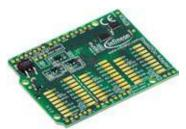
The My IoT adapter board enables designers to combine the Shield2Go boards into a system. Infineon's flexible evaluation boards are compatible with the existing solutions on the market.
