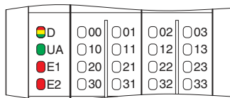
Figure 10 Local status and diagnostic indicators
