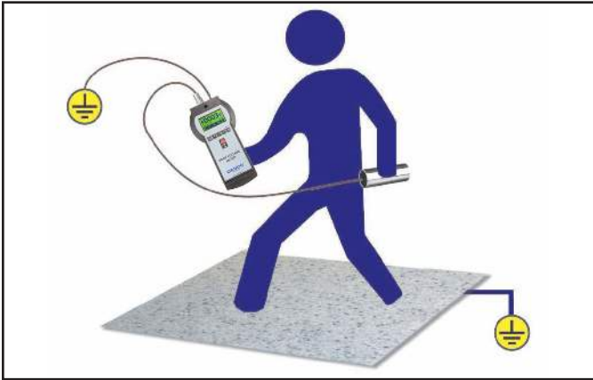
Figure 3. Setup of the Body Voltage Meter
