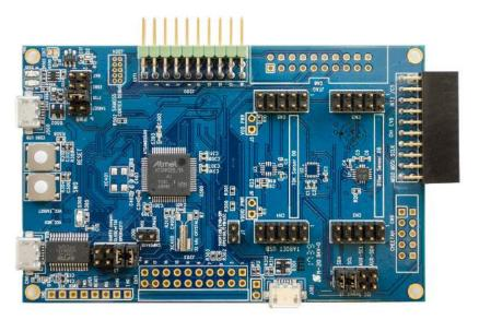
Embedded Motion Drivers (eMD) consists of a set of application programming interfaces (APIs) to configure various aspects of the platform including IAM-20680 sensor parameters such as full-scale range (FSR), output data rate (ODR), low-power or low-noise mode, Accelerometer, Gyroscope Calibration and sensor interface to host (I2C, SPI).
